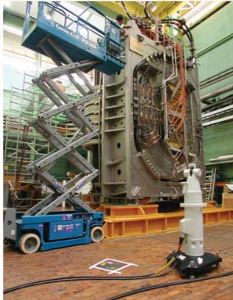
Inspection of the prototype coil for the ITER toroidal magnet
