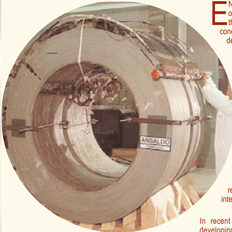
First large-dimension Nb-Ti superconducting magnet designed and built in Italy by ENEA, Europa Metalli and Ansaldo in 1980 for the SULTAN Test Facility – Villigen, Switzerland
