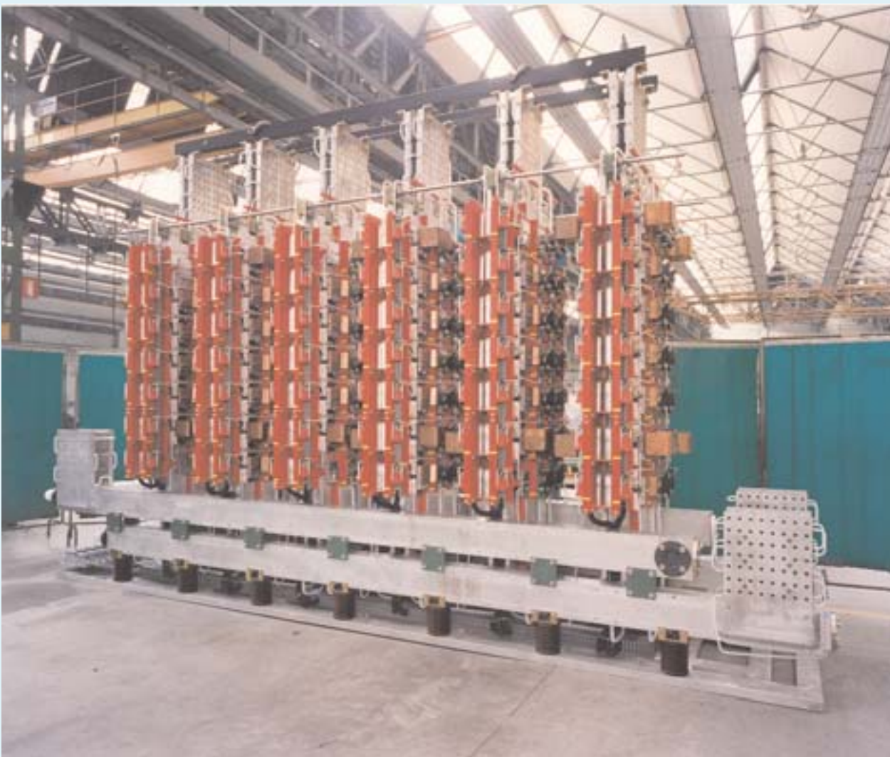
Prototype of power amplifier built at Ansaldo for ITER
