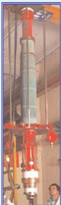
One of the gyrotrons used in the LHCD plant of FTU
