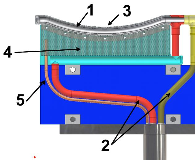
**Fig. 1.2** - The new liquid lithium limiter; 1 Mo Single structural element - 2 Inlet and outlet liquid cooling system tubes - 3 CPS (Capillary Porous System) 4- Li reservoir 5- Li filling tube.
