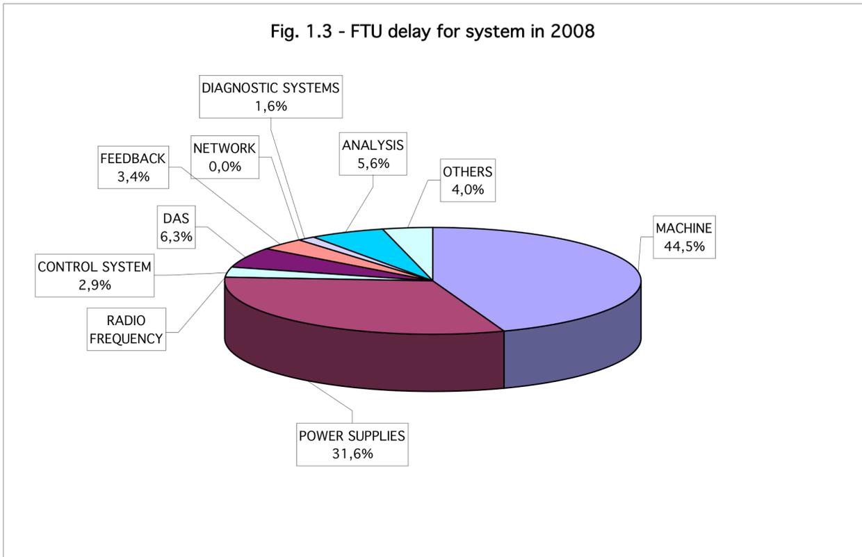
**Fig. 1.3** - Source of downtime in 2008. Machine is the greatest cause of delay with 44,5% of the total.
