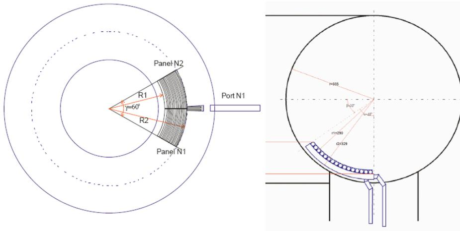
**Fig 1.1** - Top view and cross section of the panel liquid limiter for FTU
